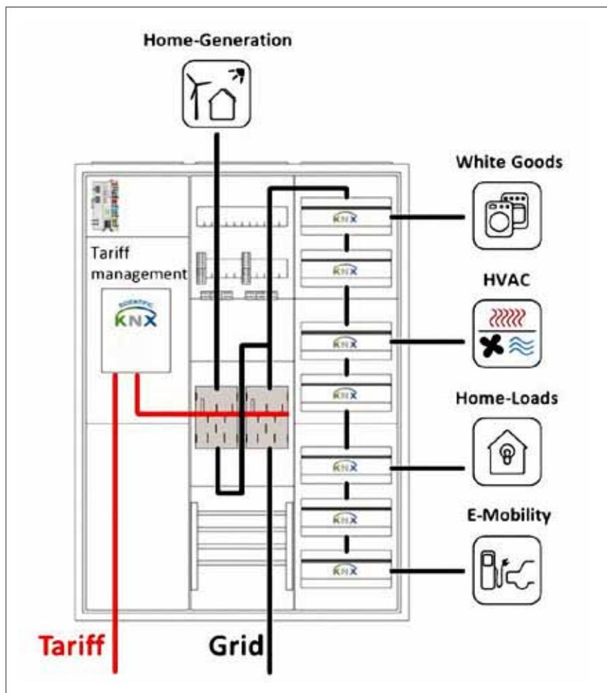
KNX main power distribution board including a metering and a distribution section. The current production of an energy generation system, as well as the consumption of the building itself, can be transmitted on KNX via the meter. KNX DIN rail modules can regulate loads in the distribution section depending on meter values. Moreover, the loads can be adapted to a tariff that was transmitted by an energy manager.
