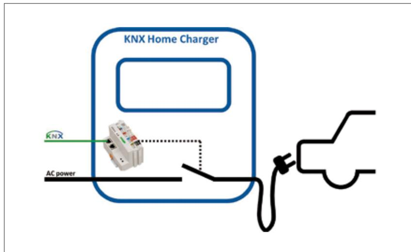
roller and, on the other hand, to enable remote starting of the charging process (closure of the charging contactor).
