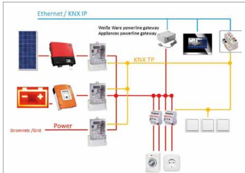
*KNX Load Management: An algorithm based on KNX PLC guarantees the optimal switching of loads and white goods in relation to the present solar power system. And thanks to simultaneous energy sub metering of the KNX actuator loads, a power buffer can also be established if required.*
