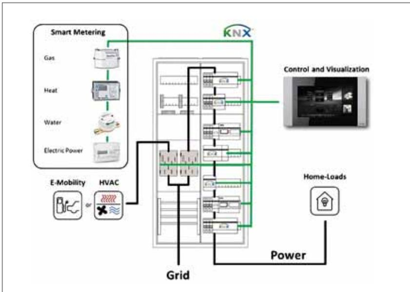
KNX provides sensors and actuators for all application domains. The diagram depicts the typical topology of a KNX installation in a main power distribution board, including the electric meter for measuring consumption, for example, as well as HVAC applications or electromobility.
